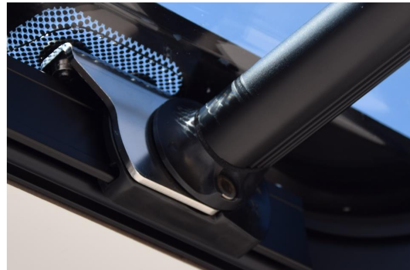
BlueSky Manual details: slider with excenter and lifting bracket
